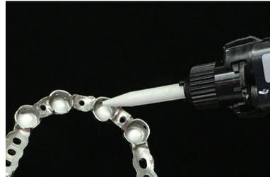
*Flow a small amount of pick up material into the substructure receiving areas*
